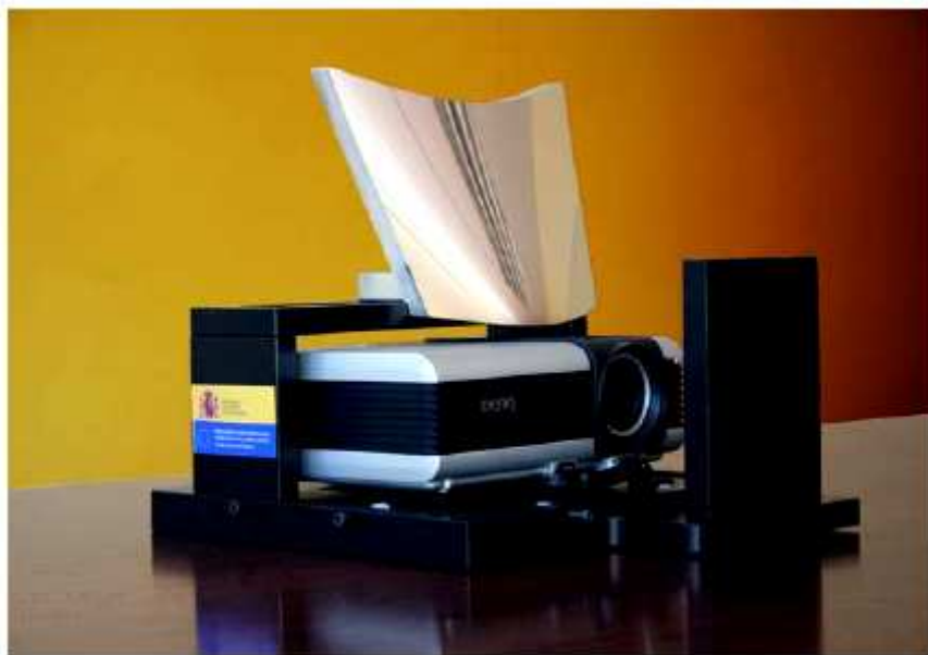
FIG. 8. Prototype of SMS ultra-wide-angle projection mirror with conventional slide projector.
