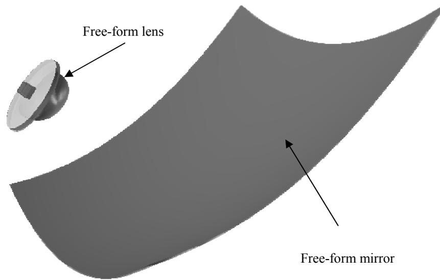
Figure 4 Isometric view of designed XR concentrator
