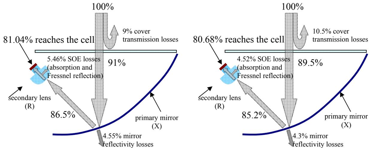
Figure 13 Graphical presentation of the losses distribution in the system: designed (left) and measured (right) values for the parts.
