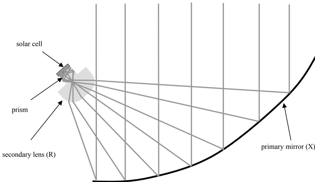
Figure 1 Cross section of an XR SMS3D concentrator
