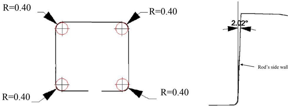
Figure 10 Measurement results of the homogenizing rod's convex curvature radii; left: homogenizing rod's exit surface; left: vertical section of the rod
