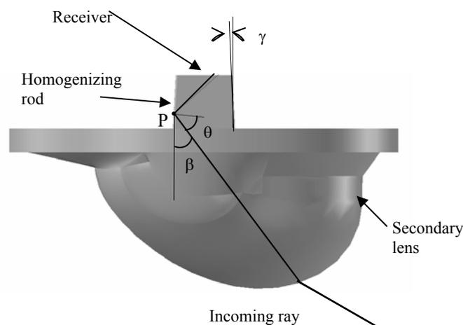
Figure 2 Secondary lens with mixing rod
