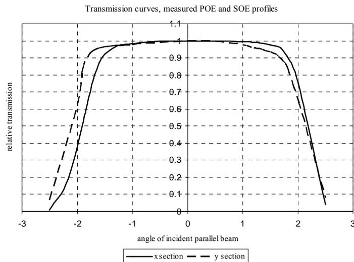
Figure 11 Simulated transmission curves of measured profiles of primary mirror and secondary lens
