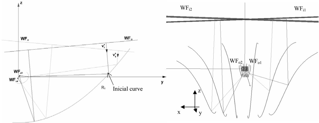
Figure 3: Schematic design procedure for the XR SMS design. Left: 2D design to create seed curve. Right: 3D design that creates SMS “chains” of points in space.
